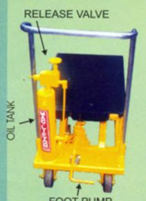
**FOOT PUMP** FOOT OPERATED SCISSOR LIFT FOR LIGHT LOADS
